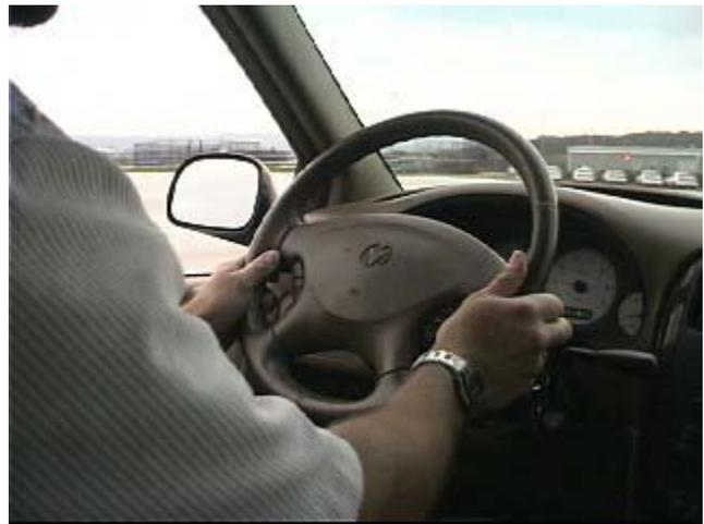
When seated in an upright position, the driver will not see the left and right sides of the vehicle when glancing at the outside mirrors. However, this adjustment adds 12 to 16 degrees additional viewing area to each side of the vehicle, provides greatest visibility to the rear of the vehicle, and reduces blind spots.
